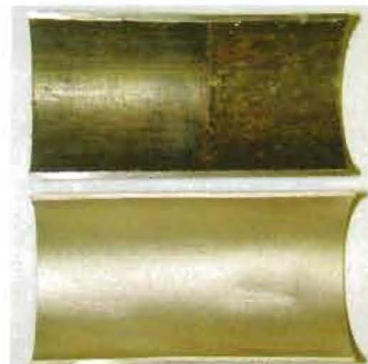
1. Condenser tube inlet where the AL6X shield had been installed is at the bottom. Note that the wooden plug could not be removed from the insert when it was extracted from the tube (top of photo)
