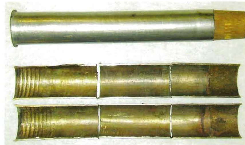
1. Condenser tube inlet where the AL6X shield had been installed is at the bottom. Note that the wooden plug could not be removed from the insert when it was extracted from the tube (top of photo)
