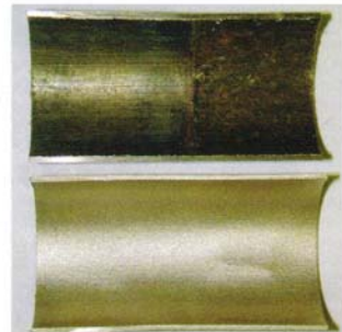
1. Condenser tube inlet where the AL6X shield had been installed is at the bottom. Note that the wooden plug could not be removed from the insert when it was extracted from the tube (top of photo)
